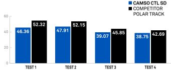
Tests on ice proved that the Camso CTL SD track is 11% more manageable on icy conditions than the competitor. To see the results on video, visit: bit.ly/1gGPY0f
