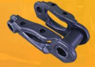
All of our track links are forged from top quality 35Cr and 40Cr carbon chromium steel. The track link body is manufactured to a hardness of HRC33~37 and the top surface of the track links are manufactured with an induction heating process to a hardness of HRC52~56. The track links are then sent into heat treatment and tempering to prevent any cracking after quenching.
