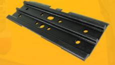
All of our track shoes are milled into a long profile from top quality manganese boron steel billet (23MnB). The profiles are then precision cut to the required length and both bolt-holes and mud-holes are punched out to accommodate for the required sizes and sent into heat treatment and tempering to prevent any cracking after quenching.
